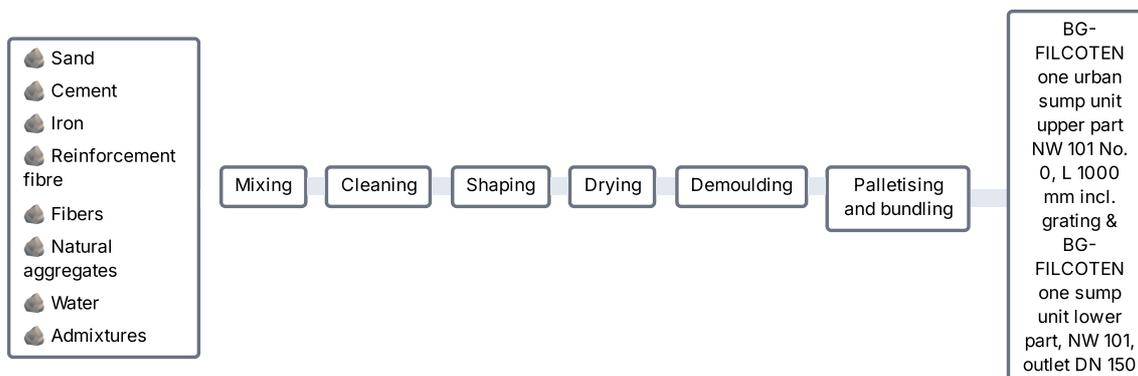
Drainage channels out of concret - FILCOTEN® HPC (High Performance Concrete) - for vehicular and pedestrian areas according to standard EN 1433
