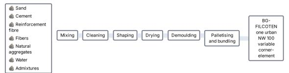
Drainage channels out of concret - FILCOTEN® HPC (High Performance Concrete) - for vehicular and pedestrian areas according to standard EN 1433
